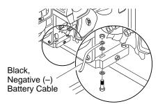
Figure 11 - Connecting Black, Negative (-) Battery Cable to Engine Block (Model RGH7500AIE Shown)
